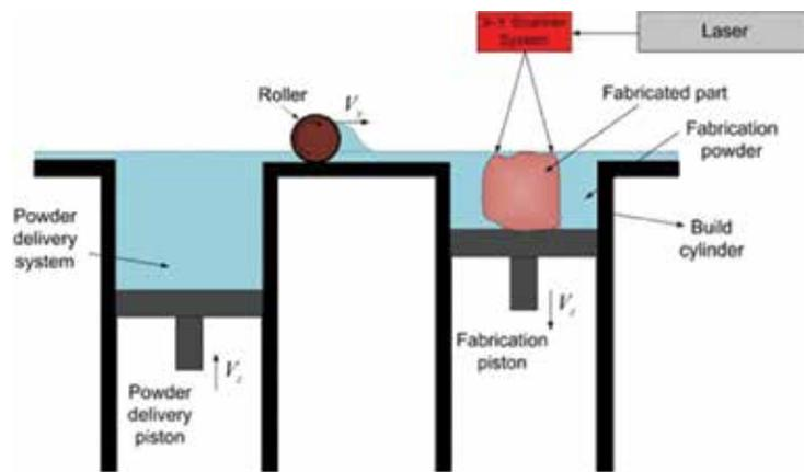
Fig. 3: Selective Laser Sintering (SLS)
